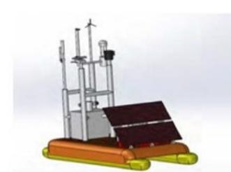
by IUSSTF, it is a collaborative project between IIT Kanpur and WHOI, USA to develop a low-cost, multi-parameter, water quality platform that will have several in-house developed sensors and auto-sampling capability for durable and reliable real-time monitoring of Indian Rivers.
