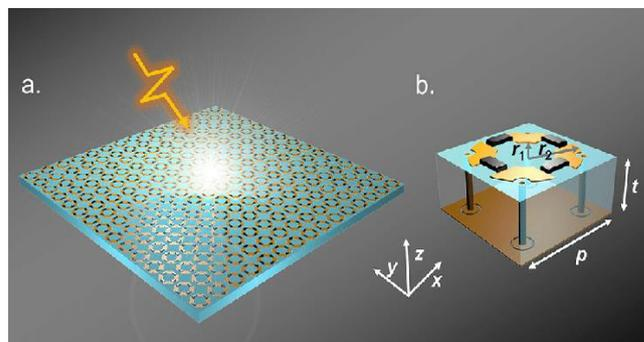
miniaturization, wider adaptability, and increased effectiveness. Intended applications for the metamaterial absorber include emitters, photodetectors, sensors, spatial light modulators, wireless communication, and use in solar photovoltaics and thermophotovoltaics.
