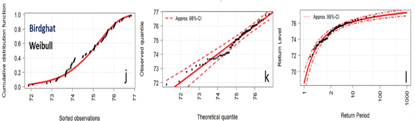
Figure 2: Fitting distributions to peak stage level: CDF plots, Quantile–Quantile plot and return level corresponding to different return periods
