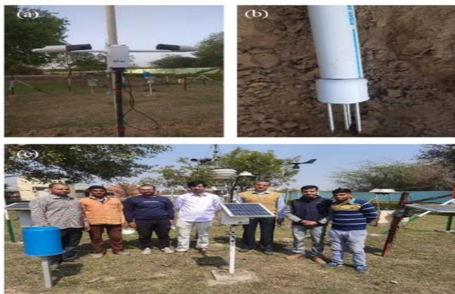
Figure 1. Sensors installed at IIT Kanpur – (a) visibility sensor, (b) soil moisture sensor and (c) automatic weather station
