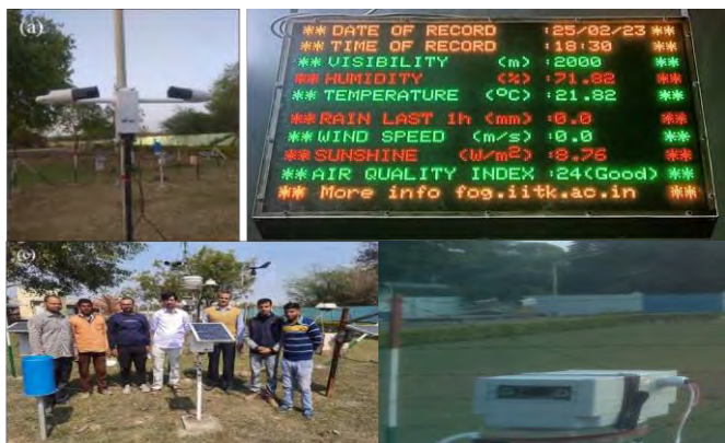
Figure 1. Sensors and display board installed at IIT Kanpur – (a) visibility sensor, (b) real-time display board in the faculty building, (c) automatic weather station, and (d) low-cost optical sensor for fog detection.
